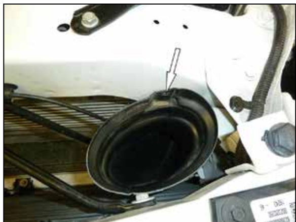
7. Remove the plastic retaining clip that secures the fresh air intake duct to the core support, then pull the duct forward to disengage it from the factory air filter housing.
