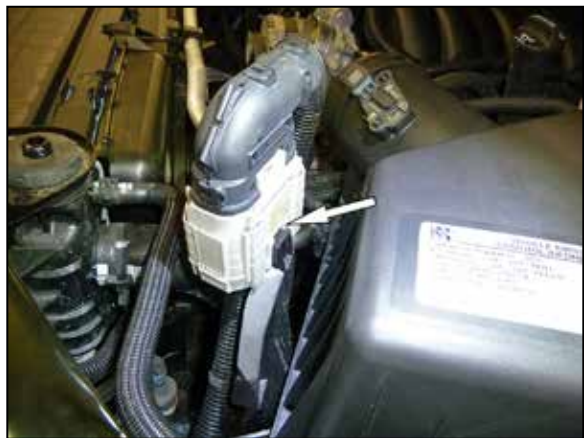
8. Using a small 90° pick or similar tool, release the locking tab that secures the wiring harness bulk connector to the air filter housing and then unhook the connector from the housing.
