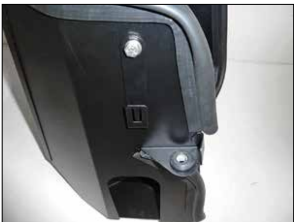
12. Install the provided wiring connector mounting bracket onto the heat shield using the provided hardware. Install the factory mounting grommet into the heat shield as shown.
