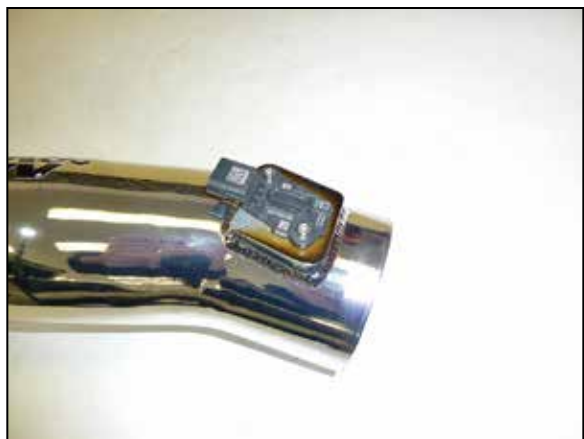
21. Remove the mass air sensor from the factory housing. Install the mass air sensor into the K&N® intake tube and secure with the provided hardware.
