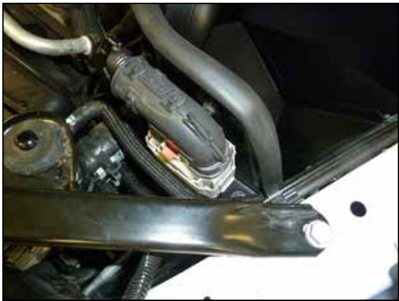
15. Connect the wiring bulk connector onto the bracket installed onto the heat shield.
