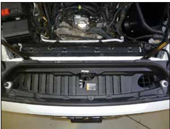
16. Reinstall the radiator valence and secure with the ten factory clips.
