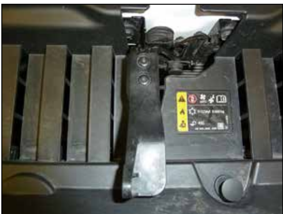
17. Reinstall the hood release arm and secure with the factory hardware.
