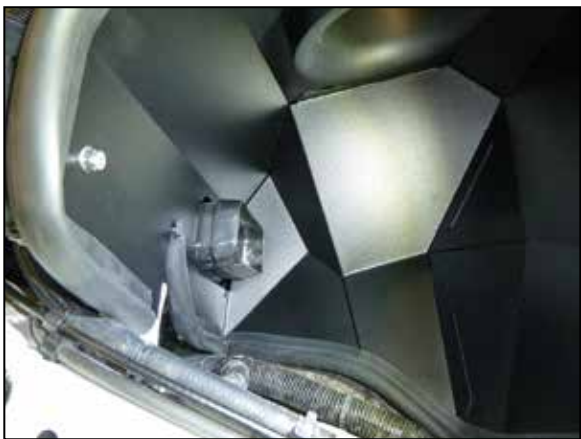
14. Install the heat shield assembly into the vehicle so the mounting grommet slides into the factory mounting hole. Slide the fresh air intake scoop into the opening in the heat shield and resecure to the core support with the factory clip. Secure the heat shield with the factory nut removed in step #9.
