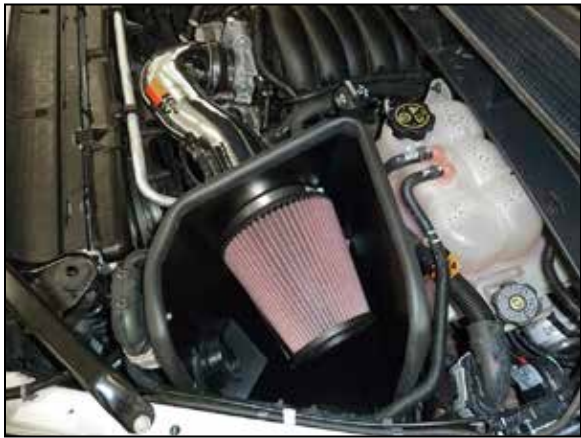
26. Install the K&N® air filter onto the adapter and secure with the provided hose clamp.
