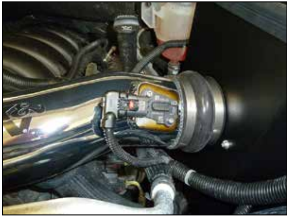
25. Connect the mass air sensor electrical connection.
