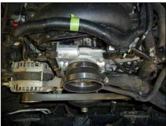
19. Install the provided reducer coupler onto the throttle body and secure with the provided hose clamp. NOTE: On 5.3L equipped vehicles use coupler #KITRDCR23, on 6.2L vehicles use coupler #KITRDCR19.
