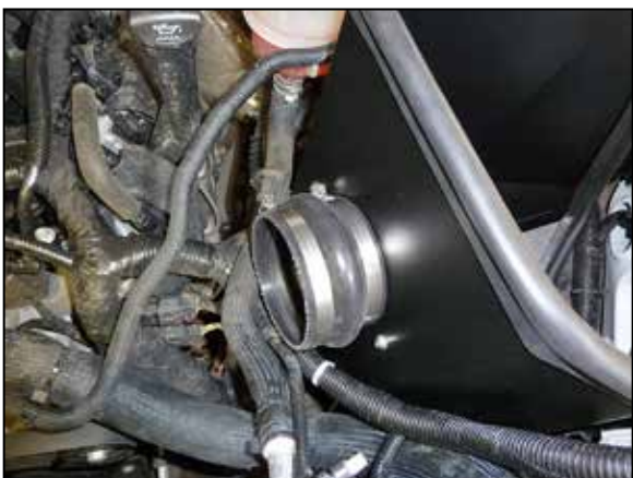
18. Install the provided hump coupler onto the filter adapter and secure with the provided hose clamp.
