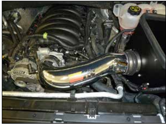
22. Install the intake tube into the coupler at the filter adapter and then into the coupler at the throttle body, adjust the tube for best fit and then secure with the provided hose clamps.
