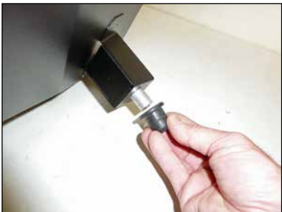
13. Install the provided grommet mount onto the heat shield using the provided hardware and then install the factory mounting grommet onto the mount as shown.
