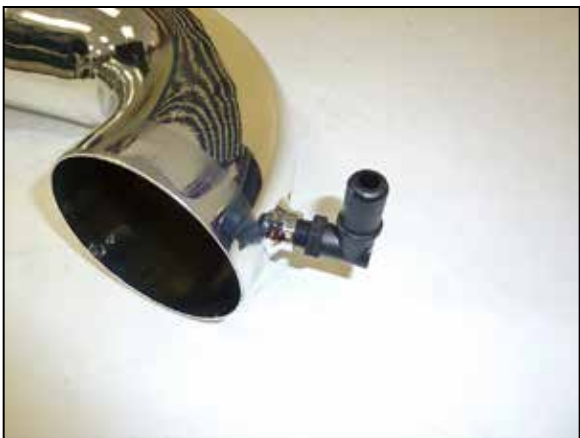
20. Install the provided 90° quick connect fitting into the K&N® intake tube as shown.
