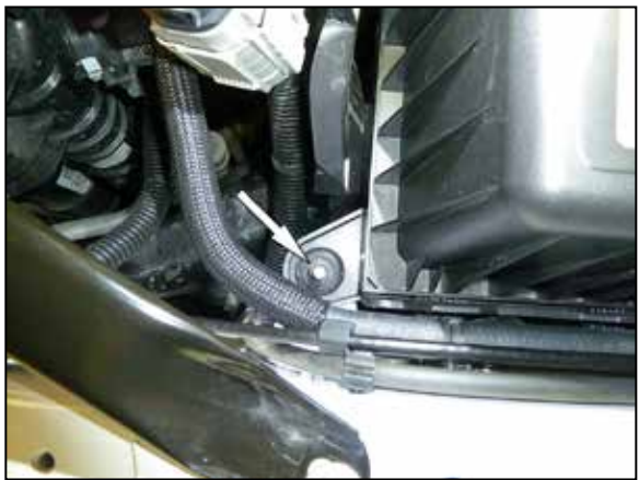
9. Remove the nut that secures the air filter housing. Unhook the wiring harness from the filter housing and then remove the air filter housing from the vehicle.
